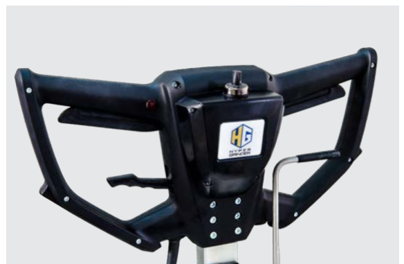
Speed regulator on the handle to maximize performance in any situation (optional).
