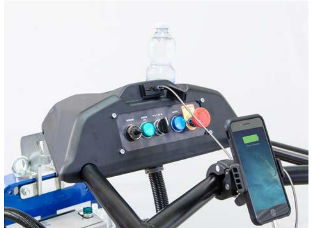
NEW DASHBOARD (STANDARD) WITH CUP HOLDER AND 2 USB SOCKETS.
