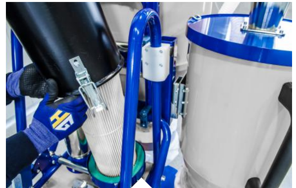
Large HEPA filter.
